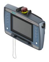
SIMATIC HMI KTP700F Mobile Arctic, (extended operating temperature range), 7.0" TFT display, 800x 480 pixel, 16m colors, key and touch operation, 8 function keys, 1x PROFINET/Industrial Ethernet interface, 1x multimedia card, 1x USB, 1x touch pen, keyswitch, acknowledgement button, emergency shutdown/stop button, configurable from WinCC Comfort V15 SP1
