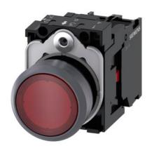
Illuminated pushbutton, 22 mm, round, plastic with metal front ring, red, pushbutton, flat, momentary contact type, with holder, 1NC, LED module with integrated LED 110 V AC, screw terminal, with laser labeling, upper case
