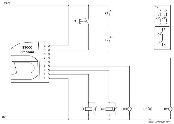
S3000 Standard in conjunction with relays/contactors
