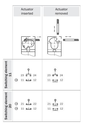
Switching element 11: 1 positive action N/C contact + 1 N/O contact
