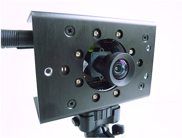
Figure 33: DME 660 tripod mounting
