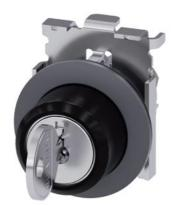
RONIS key-operated switch, 30 mm, round, Metal, matte, front ring for flush installation, lock number SB30, with 2 keys, 3 switch positions I-O-II, latching, actuating angle  $2x45^{\circ}$ , 10:30h/12h/13:30h, Key removal I+O+II, possible special locks: SB31, 421, 455, Z=50-unit packaging
