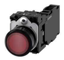
Illuminated pushbutton, 22 mm, round, plastic, red, pushbutton, flat, momentary contact type, with holder, 1 NO+1 NC, LED module with integrated LED 24 V AC/DC, screw terminal, Z=20-unit packaging
