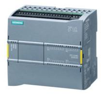
SIPLUS S7-1200 CPU 1214FC DC/DC/relay based on 6ES7214-1HF40-0XB0 with conformal coating, -25...+55  $^{\circ}$ C, compact CPU, DC/DC/relay, onboard I/O: 14 DI 24 V DC; 10 DQ relay 2 A; 2 AI 0-10 V DC, power supply: DC 20.4-28.8 V DC, program/data memory 125 KB
