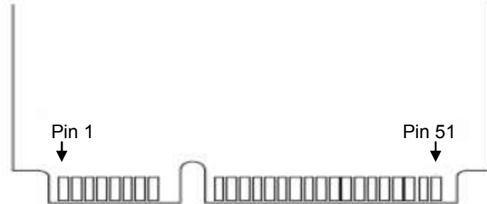
Figure 1-2 Apacer mSATA H1-M pin assignment
