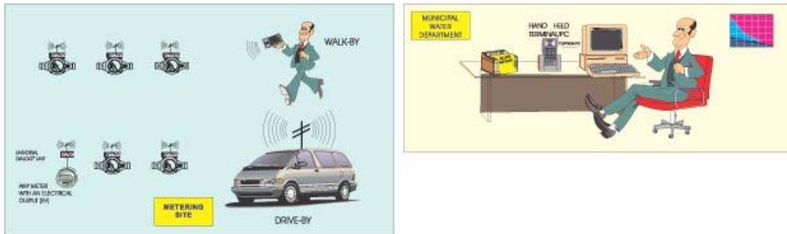
Figure 6–5. Overview of the AMR System
