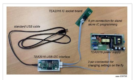
Figure 8. Connecting the setup
