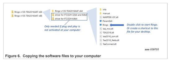
For the Ringo software to work, the FT232H driver for the USB-I<sup>2</sup>C interface must be installed. When the interface is connected via USB for the first time, this installation happens automatically. If the driver is not installed automatically, use the included drivers to install it manually (a video on the get started page shows how to install the driver
