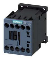
Power contactor, AC-3 12 A, 5.5 kW / 400 V 2 NO + 2 NC 125 V DC 4-pole Size S00 screw terminals
