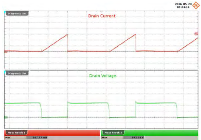
Figure 70 – 90 VAC, 48 V LED Load. Upper: I_{DRAIN} , 100 mA / div. Lower: V_{DRAIN} , 50 V / div., 5 \mu s / div.
