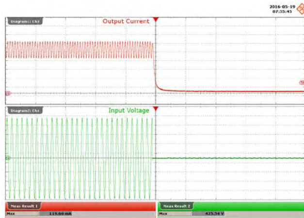
Figure 68 – 230 VAC, 48 V LED, Output Fall. Upper: I_{OUT} , 40 mA / div. Lower: V_{IN} , 100 V / div., 100 ms / div.
