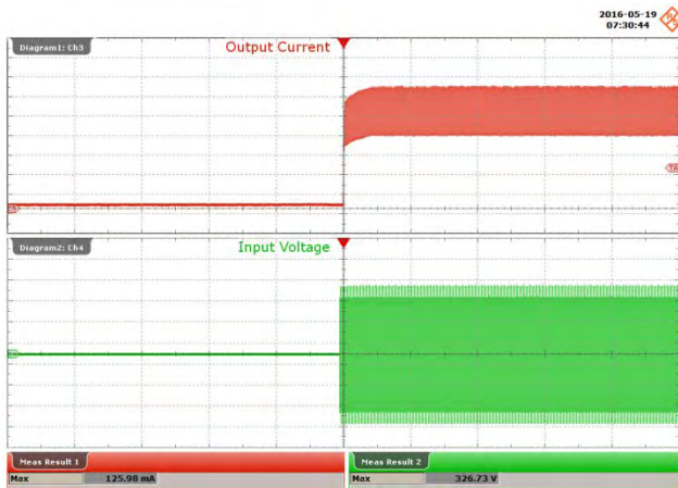
Figure 61 – 230 VAC, 48 V LED, Output Rise. Upper: I_{OUT} , 40 mA / div. Lower: V_{IN} , 100 V / div., 1 s / div.
