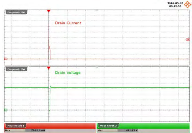
Figure 80 – 300 VAC, 48 V LED Load. Upper: I_{DRAIN} , 100 mA / div. Lower: V_{DRAIN} , 100 V / div., 4 \mu s / div.
