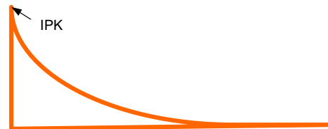
Figure 47. Input Charge Inrush Current
