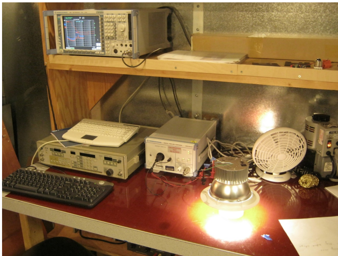
Figure 72 – EMI Test Set-up.
