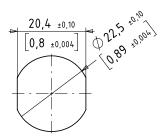
The SENSORswitch is secured against rotation by the illustrated
