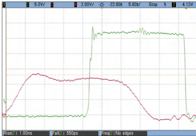
Figure 4: Typical Waveforms for V_{IN} = 28\text{ V} to 3.3\text{ V}/4\text{ A} (5 MHz) Buck converter CH2: ( V_{OUT} ) Switch node voltage — CH4: V_{PWM} Input voltage
