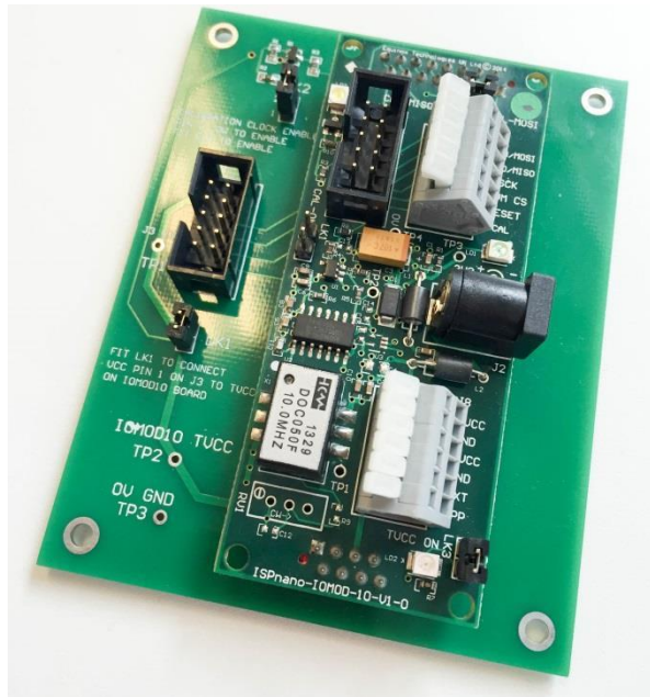
Figure 2: IOMOD10-CB1 with IOMOD10 calibration board
