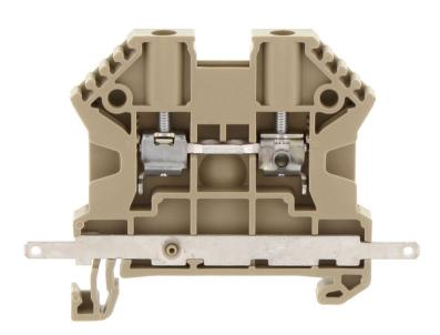
Feed-through terminal, Screw connection, Mounting type: Mounting rail TS 35/7.5, Rated cross-section: 2.5 mm², Width: 5 mm, Colour: Beige
