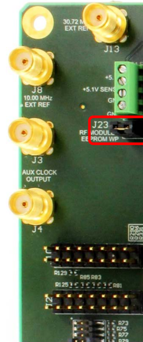
Figure 23. EEPROM Write Protect Header RF A
