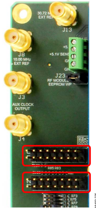
Figure 25. RF A Debug Header Pins
