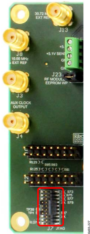
Figure 27. JTAG Debug Header Pins
