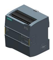
SIMATIC S7-1200, CPU 1212FC, compact CPU, DC/DC/relay, onboard I/O: 8 DI 24 V DC; 6 DO relay 2 A; 2 AI 0-10 V DC, Power supply: DC 20.4-28.8V DC, Program/data memory 100 KB
