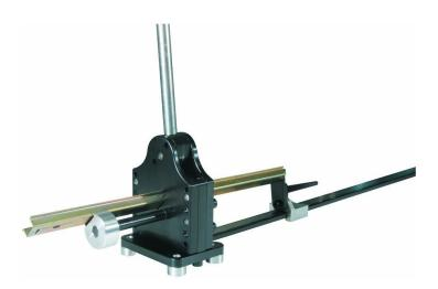
The TS-PS eco DIN rail cutter is a manual tool designed for cutting DIN TS 35 rails into shorter sections. The TS-PS eco has a quiet and quick cutting process which leaves no burrs on the rail. The result is a fine, straight cut that does not result in any bending of the rail. The tool can be attached to a work bench or mounted at a workstation.
