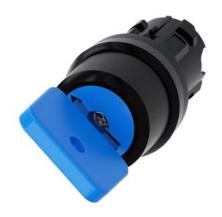
Key-operated switch O.M.R, 22 mm, round, plastic, lock number 73038, blue, with 2 keys, 2 switch positions O<I, momentary contact type, Actuating angle 45°, 10:30h/12h, key removal O, with laser labeling, lower case
