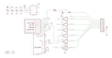
For the level shifter we use the CD74HC4050 which has a typical propagation delay of  $^{\sim}10 ns$
