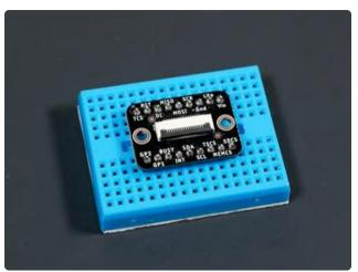
To begin inserting an EYESPI cable to an FPC connector, gently lift the FPC connector black latch up.
