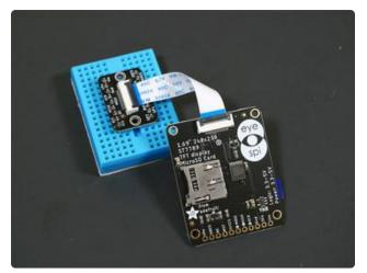
Repeat this process for the FPC connector on your display. Again, ensure that the blue stripe on either end of the cable is facing up.
