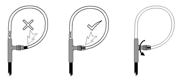
Once the free end of the coil is fully engaged in the ferrule, turn the ferrule lock nut to lock the coil end in position.
