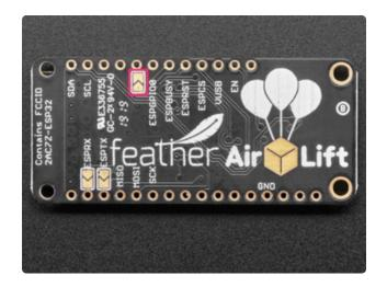
Note: These pin definitions leave the the ESP32's GPIO0 pin undefined (-1).
