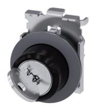
RONIS key-operated switch, 30 mm, round, Metal, matte, front ring for flush installation, lock number SB30, with 2 keys, 2 switch positions O<I, momentary contact type, Actuating angle 45°, 10:30h/12h, key removal O, possible special locks: SB31, 421, 455, with laser labeling, upper case and lower case, always upper case at the beginning of the word
