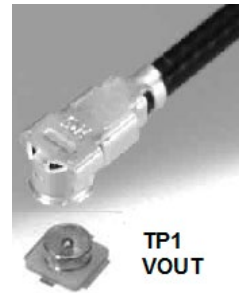
Figure 4. Technique for Measuring Output Ripple and Step Response with a Low Inductance Connector (Not Supplied)
