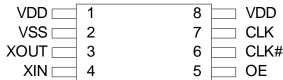
Figure 1. Pin Diagram – 8-Pin TSSOP
