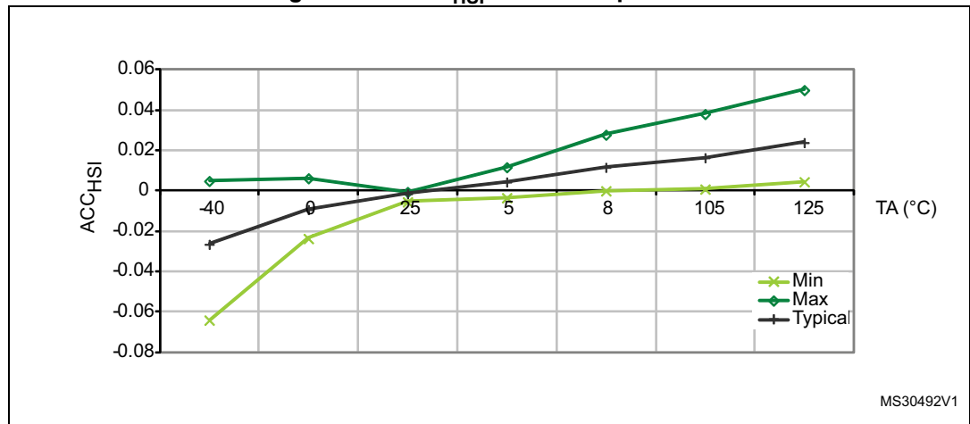
Figure 27. LACC_{HSI} versus temperature
