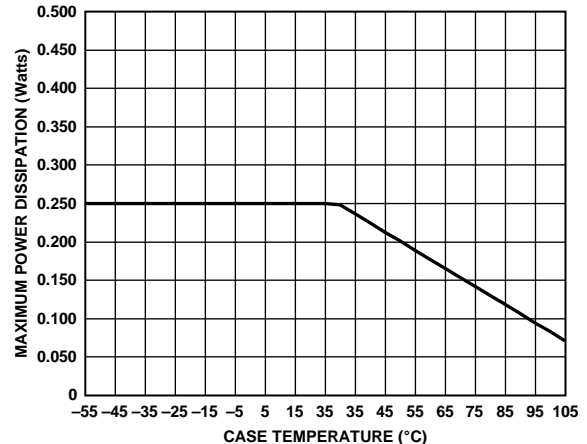
Figure 4. Maximum Power Dissipation vs. Case Temperature
