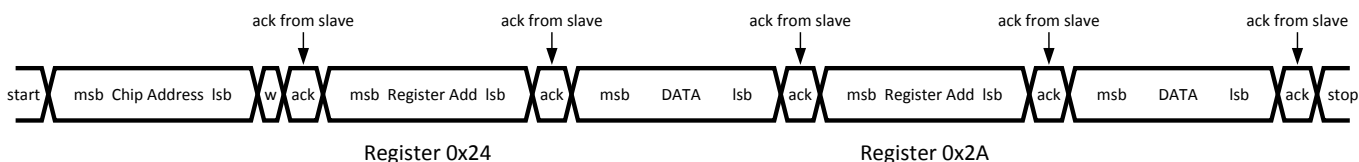
Figure 23. Multi-Byte I 2 C Command
