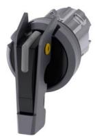
Illuminable selector switch, 22 mm, round, collar, metal front ring, metal matte, black, Selector switch long, 3 switch positions I-O-II, latching, actuating angle  $2x45^{\circ}$ , 10:30h/12h/13:30h, can be locked in I + O, with 2 padlocks, or snap hook, shackle 5 mm, can be combined with metal holder
