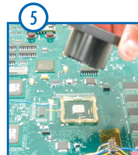
Lift to remove the Knob Tool - leaving the Frame Clip attached to the component.
