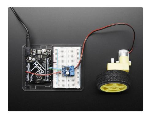
Using it is super simple. Connect your motor to the OUT terminal block. Power the board with 6.5-45VDC power on VMotor and provide the H-bridge input control on IN 1 and IN2. You can even PWM the inputs and the driver chip will do the right thing.
