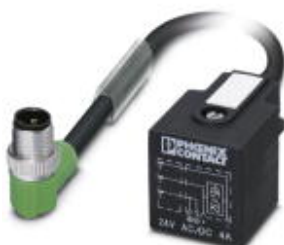
Sensor/Actuator cable, 3-position, PUR, Black RAL 9005, Plug angled M12, on A valve plug, with 1 LED
