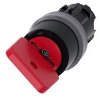
Key-operated switch O.M.R, 22 mm, round, plastic with metal front ring, lock number 73037, red, with 2 keys, 2 switch positions O-I, latching, actuating angle 90°, 10:30h/13:30h, key removal O+I, with laser labeling, upper case and lower case, always upper case at the beginning of the word
