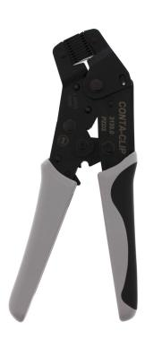
Crimping tool for crimping wire-end ferrules with and without plastic collars. Cross-section range: 0.5-6 mm² (AWG 2-10). Easy to use, Auto-lock for proper and complete crimping, Wires fed in from the front, Self-opening with built-in spring.
