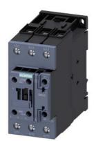
Contactor, AC-3, 37 kW / 400 V, 1 NO + 1 NC, 110 V AC, 50 Hz / 120 V, 60 Hz, 3-pole, Size S2, screw terminal Upright mounting position
