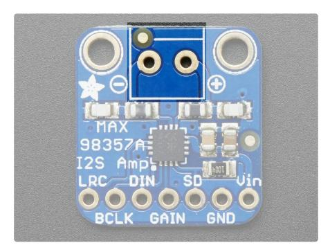
This amplifier is designed to drive moving coil loudpeakers only. Speaker impedence must be  $4\Omega$  or more. The output signal is a 330KHz PWM square wave with a duty cycle proportional to the audio signal. The inductance of the speaker coil serves as a low-pass filter to average out the high-frequency components. Do not try to use this as a pre-amplifier.
