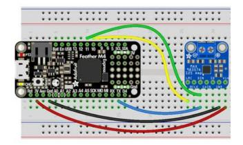
Connect VIN on the breakout to 3V on the board.
