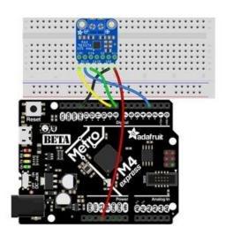
Connect VIN on the breakout to 3.3 on the board.
