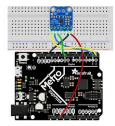
Connect VIN on the breakout to 3V/3.3 on the board.
