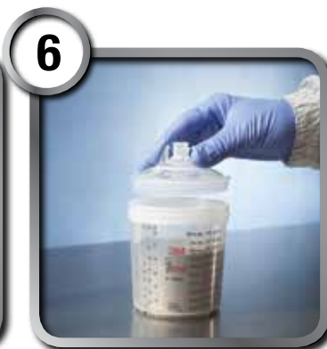
Take a lid (with built-in filter) from wall dispenser and snap into the 3M™ PPS™ cup/liner.
