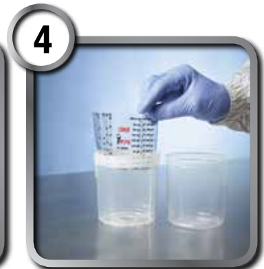
If not using a scale to measure, insert 3M™ PPS™ mix ratio film into cup before inserting liner in order to measure the paint according to paint manufacturer's guidelines.
