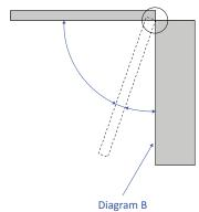
The damper torque becomes larger, preventing the lid from closing completely
