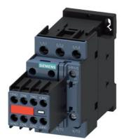
Power contactor, AC-3 25 A, 11 kW / 400 V 2 NO + 2 NC, 110 V AC, 50 Hz, 120 V, 60 Hz, 3-pole, Size S0, Screw terminal Captive auxiliary switch
