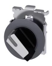
Selector switch, illuminable, 30 mm, round, Metal, matte, white, selector switch, short, front ring for flush installation, 2 switch positions O<I, momentary contact type, Actuating angle 45°, 10:30h/12h, with laser labeling, upper case and lower case, always upper case at the beginning of the word
