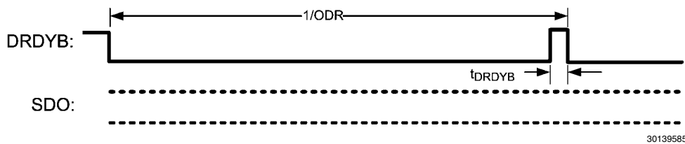
FIGURE 21. DRDYB Behavior for an ADC_DOUT not Read
