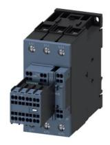
power contactor, AC-3 40 A, 18.5 kW / 400 V 2 NO + 2 NC, AC / DC 48-80 V, with varistor, 3-pole, Size S2, Spring-type terminal
