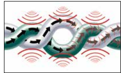
Illustration 1: Example of Non-Bonded-Pair. As cable is stretched and pulled, pairs begin to separate, causing a degradation in signal quality.
