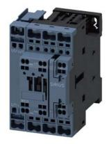
Contactor, AC-1, 50 A/400 V/40 °C, S0, 4-pole, 230 V AC, 50/60 Hz, 1 NO+1 NC, Spring-type terminal
