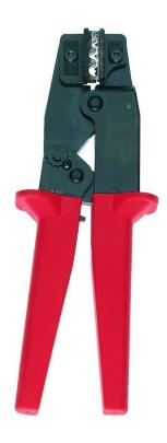
Crimping tool for non-insulated crimp lugs in flat spade shape. Easy to use, Auto-lock for proper and complete crimping, Wire can be fed in from the side, Self-opening with built-in spring.
