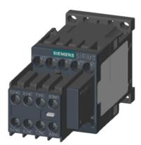
Contactor relay, 4 NO + 4 NC, 120 V AC, 50 / 60 Hz, Size S00, screw terminal, 2 NO + 2 NC basic unit / EN Varistor plugged on
